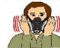
NEGATIVE PRESSURE FIT CHECK Block ends of cartridges with hands. Inhale. If mask caves in, you have a tight fit.
